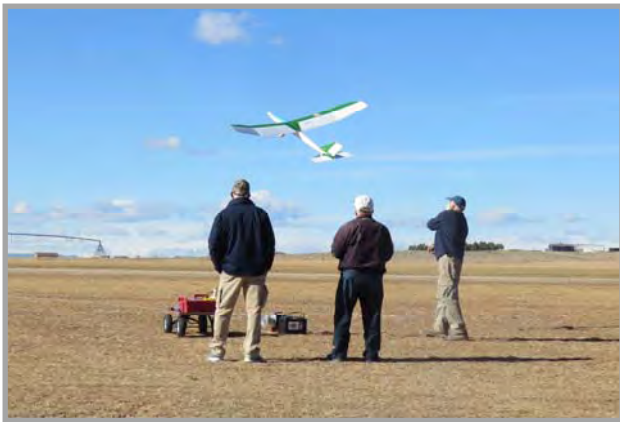
“Some gliders are hand-launched while others can be launched by a winch and cable.”
