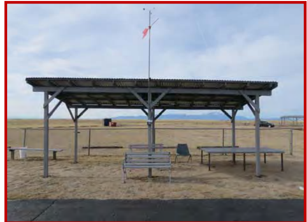
“Installed on the middle post, the wind speed indicator also has a wind arrow, giving a general direction of the winds.”
