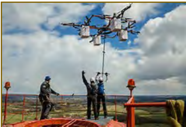
“The 28 rotor drone is capable of lifting 100 kilos or 220 pounds.”
