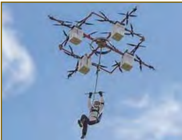
“The 28 rotor drone is capable of lifting 100 kilos or 220 pounds.”
