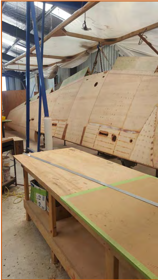
"A view of the Mosquito wing section, (54' 2" ws) all wood, just like the original Mosquitos."
