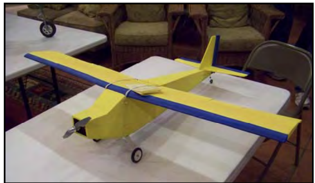
“Tom decided to try his hand at building his first plans-built airplane. So he printed the plans out of the October issue of the AMA magazine, called the Coyot-E. It is electric powered, running off a 3-cell battery. Tom had completed 3 flights on his successful project.”
