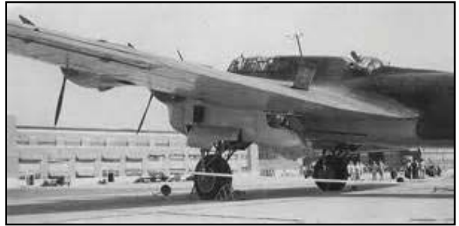
"The above photo shows the unusual gun position at the rear of each inboard engine nacelle. The gunner could crawl through the wing to get to the gun while in flight or enter through an upper hatch while on the ground."
