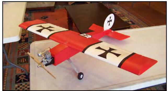
"Tom brought to the club meeting his new hybrid Stick. On the outside it looks like a glow 2-stroke engine. But on the inside it is actually powered by a electric motor running off a 3 cell battery. The drive shaft runs through the plastic engine."
