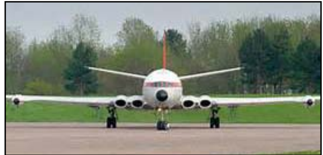
"The Comet featured an aerodynamically clean design with four De Havilland Ghost turbojet engines buried in the wings."
