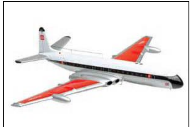
"The Comet featured an aerodynamically clean design with four De Havilland Ghost turbojet engines buried in the wings."
