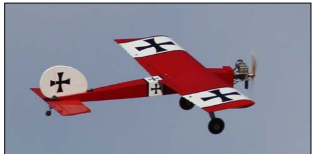
"Powered by a DLE-55 gas engine, the winds didn't bother this 82" ws plane too much."
