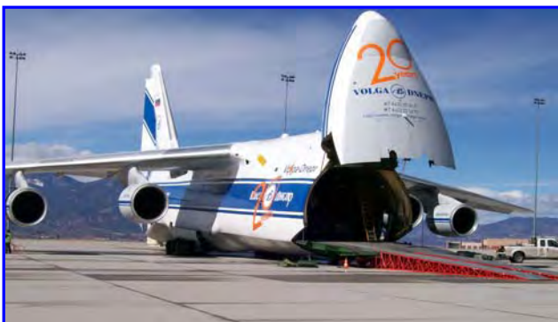
"The Condor has the same capabilities as the USAF C-5, to include front nose lift and front & rear kneeling."
