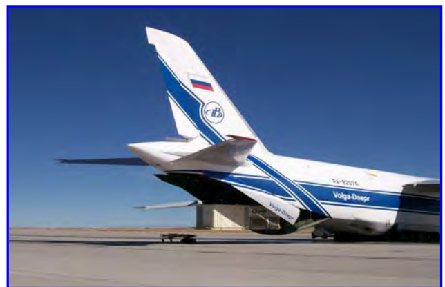
"Rear view of the Condor. One unique feature that the Condor has that the C-5 does not have, a heavy lift hoist system built in the ceiling that extends from the rear of the plane, positioning over the cargo, hooks up to the cargo, then easily lifts the cargo back into the plane."
