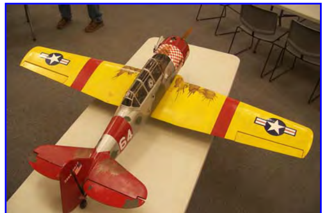
"Duane brought in his battered AT-6 complete with bullet holes, oil leaks and fire damage. Duane said this AT-6 is a 20-year old kit that has been rebuilt several times. In it's latest rebuilt upgrade, it now has an OS .75AX engine and flaps. The plane has not flown yet."
